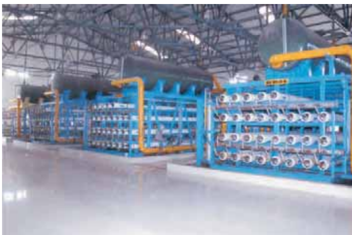
Sea water desalination plant (reverse osmosis)
