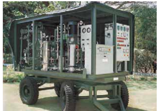
Trailer mounted reverse osmosis system with pretreatment for army camps
